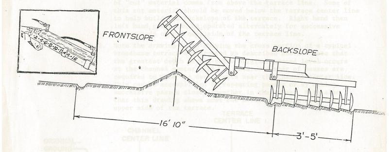
This step is similar to STEP II for constructing narrowbase terraces; however, it must be repeated more for broadbase terraces because of the greater width of the terrace. Construction of broadbase terraces will necessarily take longer than construction of narrowbase terraces.
