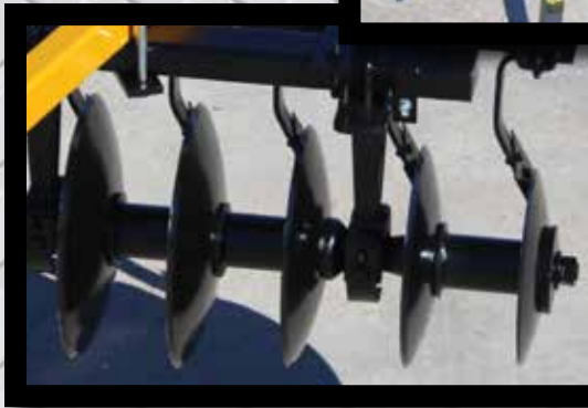
Above: Diminishing blades on the rear gang and feathering blades provide a smooth, even cut.
