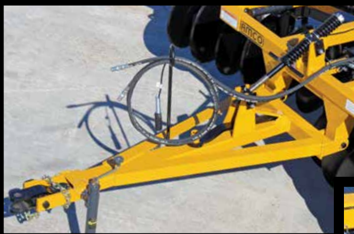
Above: Front to rear leveling spring allows easy adjustment in the field. The standard tongue jack and gang bolt wrench both fit in place on the tongue during operation. A 4" x 8" (3,000 PSI) hydraulic cylinder with hoses to tractor is also standard equipment.
