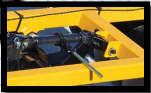
Below: Transport lockout pin ensures safe road travel.
