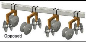
Staggered: Front blades work with back in staggered setup for extreme residue management. Opposed: Front blades opposed to back for normal conditions.
