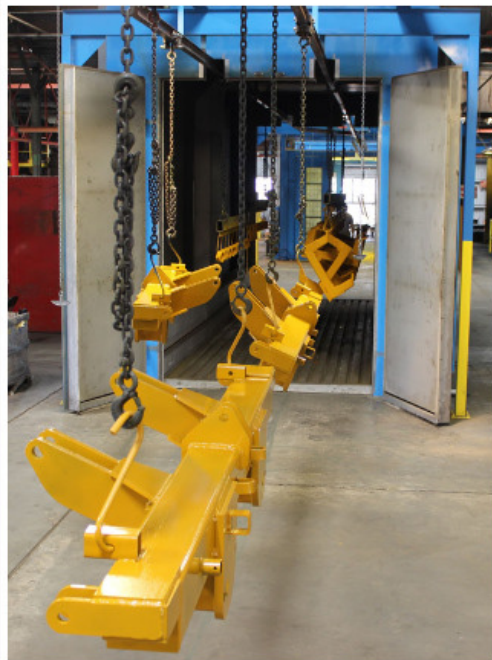
AMCO equipment parts pass through the curing oven after being powder coated. They then cool off, ready for assembly.
