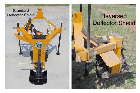
How to reverse deflector shield only on AMCO Vertical Ditchers
