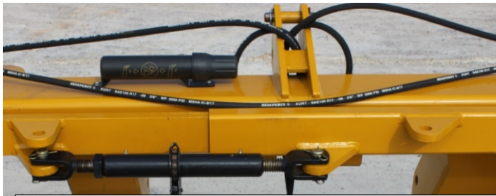
Ratchet jack for adjusting width of the levee.
