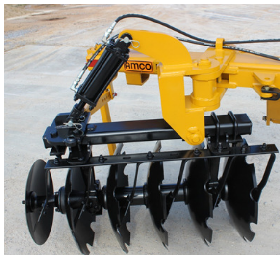
Hydraulic 10 blade gang with feathering blades
