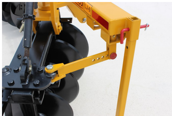
Adjustment link for changing gang angle
