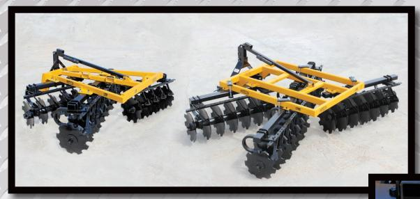
Below: AMCO's Shock Absorber Bearing Risers, standard on small- and large-frame models, allow the gang on the harrow to move upward and back to relieve shock when the disc blades encounter an obstacle in the ground.
