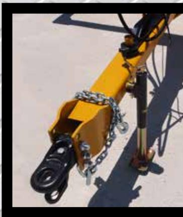
*Above: Adjustable 88.5" tongue has base hitch and conveniently stores tongue jack and gang bolt wrench during operation.*
