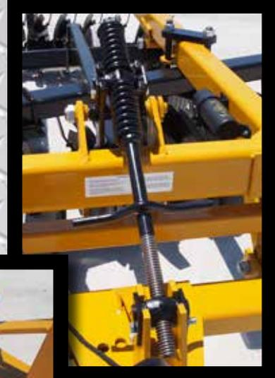
*Above: Leveling spring allows adjustments to be made for changing soil conditions.*
