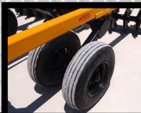
*Left: Dual wheels provide improved flotation on larger units.*
