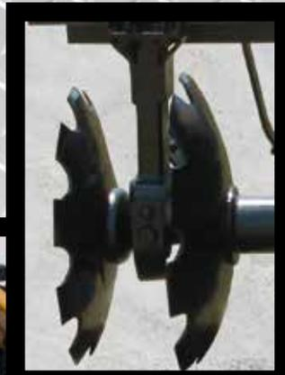
Left: Fabricated steel bearing risers are made for tough terrain and are standard equipment on J42 and F42 models.
