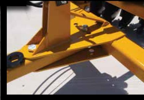
*Right: Frame clamps help assure proper frame alignment, even under the toughest field conditions.*
