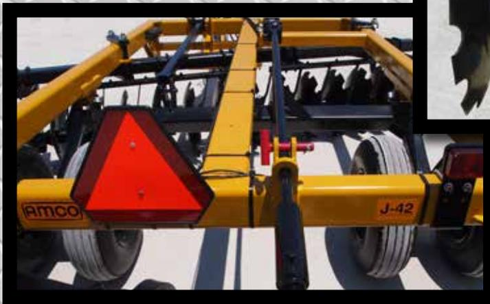
Above: Screw-type depth control combined with hydraulic cylinder maintains set cutting depth.
