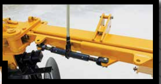
Below: The ratchet jack adjusts the cutting width, determining the overall width of the levee.
