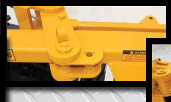
Right: Adjustment holes allow the flexibility to build extra narrow or extra wide levees.
