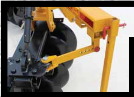
Above: Move gangs forward or back to control the cutting angle.
