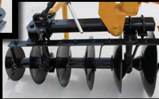
Left: Different blade configurations are available to achieve the desired levee type.
