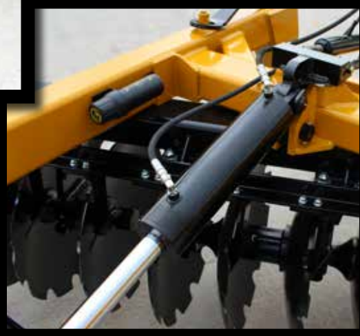
Below: Specially designed oversized 5" x 16" x 2 1/2" hydraulic cylinder lifts harrow for transport.
