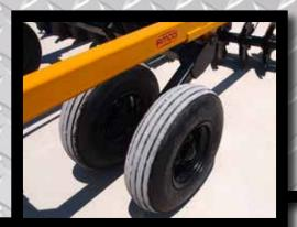
Left: Dual wheels provide improved flotation on larger units.
