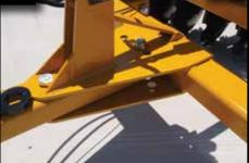
Right: Frame clamps help assure proper frame alignment, even under the toughest field conditions.
