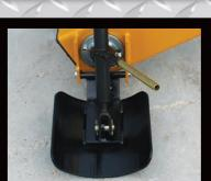
Left: Concave skid shoe with quickadjust ratchet gives better tracking for a more uniform ditch. Standard on all models.
