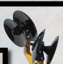
Right: Heavy-duty scrapers standard on Heavy-Duty Toolbar/Bedding Hipper combinations. Scrapers optional for Bedding Hipper Assemblies.
