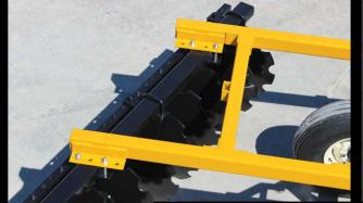
Left: Front and rear gang angle can be adjusted from 17 to 23 degrees.
