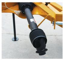
All ditcher models feature PTO drive shaft parking hook to secure PTO for storage.
