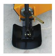
Concave skid shoe with quick-adjust ratchet gives better tracking for a more uniform ditch. Standard on all models.
