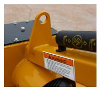
A lift hook feature on the Dominator makes it easy to attach a chain or strap for extra maneuverability when loading.
