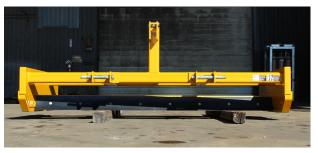
2. Loosen 4 nuts on each side of skid shoe
