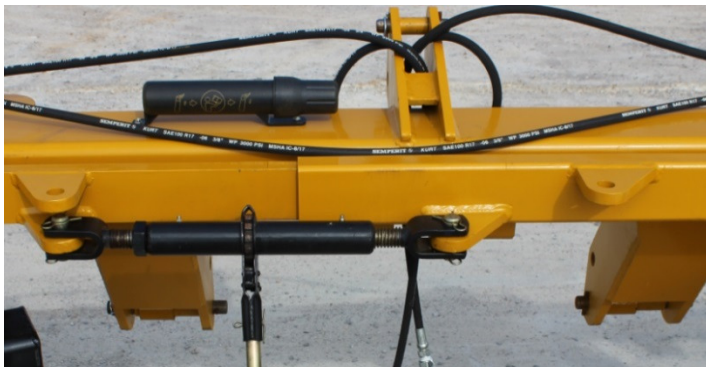
Ratchet jack for adjusting width of the levee.
