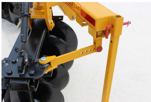
Adjustment link for changing gang angle
