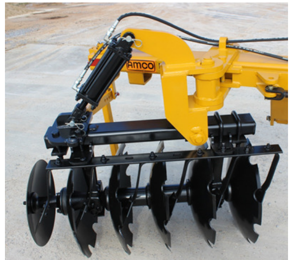
Hydraulic 10 blade gang with feathering blades
